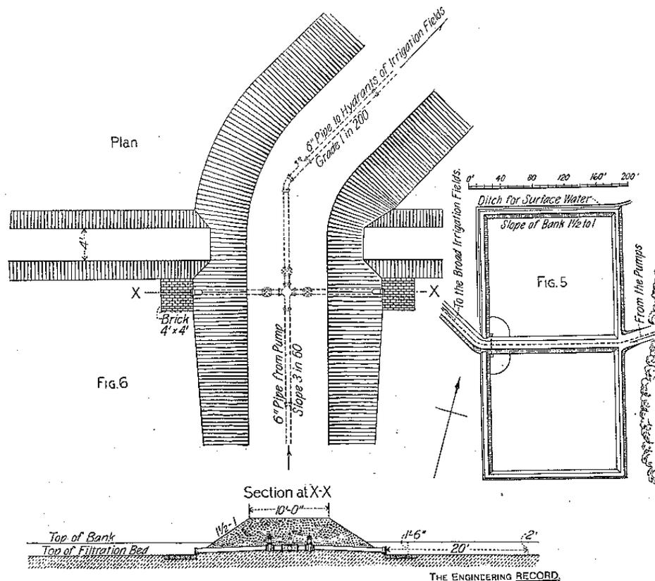
**Fig. 5:** Arrangement of filter beds, and **Fig. 6:** Details of piping (Noyes & Hazen, 1896).
