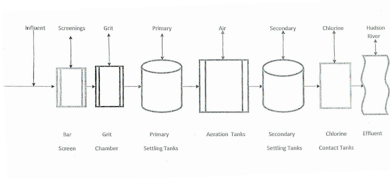
**Fig. 7:** Arlington Treatment Plant Flow Diagram (*Arlington Wastewater Treatment*)
