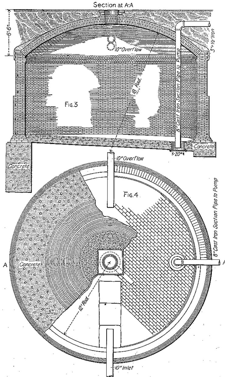
Fig. 3 and fig. 4: Receiving tanks (Noyes & Hazen, 1896).
